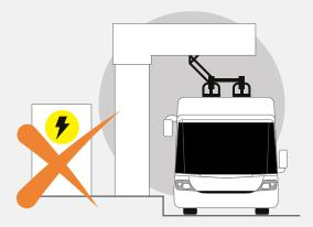
Integrated electronics requires no separate power housing and foundation
